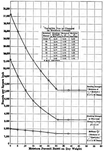
Fig. 12.—Effect of varying degrees of moisture upon the strength and stiffness of small clear pieces of western hemlock.
